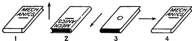
FIG. 275. Three consecutive 180-deg rotations about perpendicular axes bring a rigid body back to its starting position.
